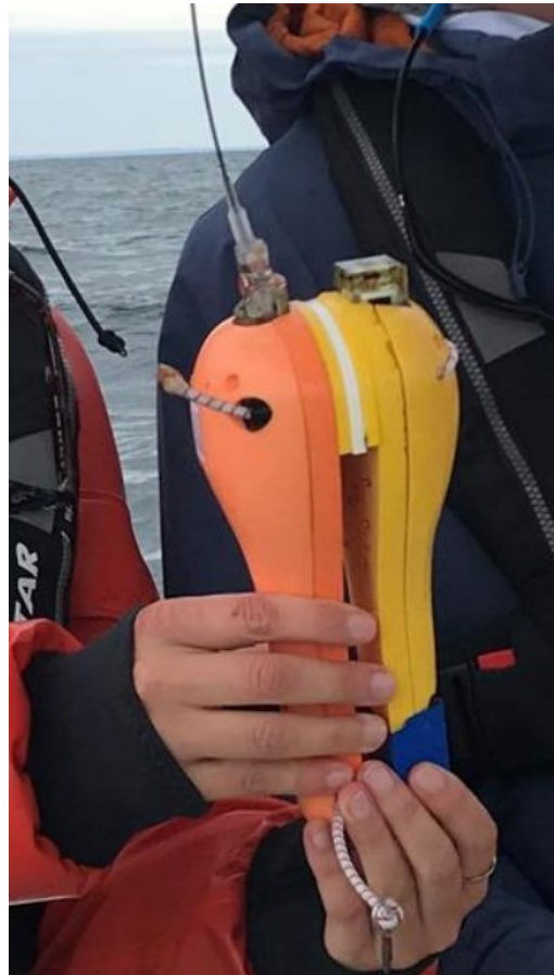
Figure 4. Package consisting of a PSAT, DST and Camera deployed on ABFT Fins in Skagerrak 2024. Photo: Henrik Baktoft ©.
